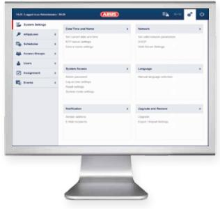
New cylinders can be assigned within the Control at any time. The configuration panel can then be used to set up the opening time and the arming function. Under System settings, an administrator can adjust all the key options for access, network and e-mail messaging, as well as date, time and language.
